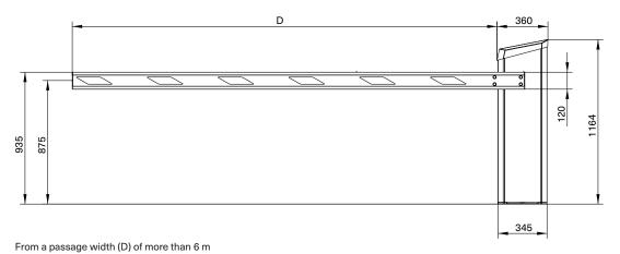
the barrier boom consists of two profiles 360
